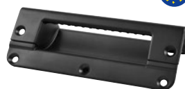
No. 30000830 ROADINGER Insert dish handle, black plastic • Cut-out 50 x 95 mm • Weight approx. 40 g • Mounting holes: d=5.0 mm
