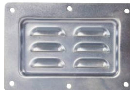
No. 30000197 ROADINGER Inlet dish, ventilation • 1 mm steel, zinc-plated • Weight: approx. 160 g • Cut-out: 126 x 74 mm • Mounting holes: d=5.1 mm
